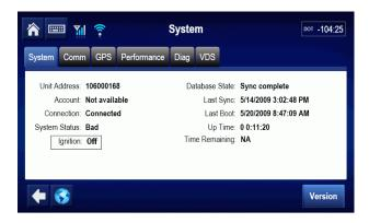
If the System Status does not change to Ignition OFF after you turn OFF the ignition, the power cable's ignition wire is most likely connected to the wrong source. Verify that the ignition wire is connected to 12VDC ignition-switched power source.
