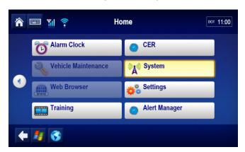
2. Tap the **System** tab. Tap the **Version** button at the bottom right to access system information about the MCP110.
