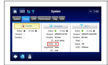
To view the RSSI value, from the Omnitracs MCP110 Home screen, touch the **System** button, then touch the **Comm** tab. The center column shows the RSSI value.
