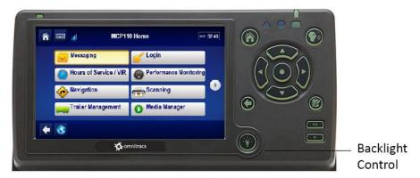
The brightness toggles the touchscreen backlighting up and down 20% for each press. When the backlight is completely OFF, the brightness control key will be in an amber color.
