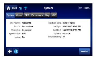
The MCP110 Unit Address is at the top of the page. The MAS also has the Unit Address written on the yellow label.
