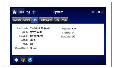
To access more detailed information concerning the GPS screen use the GPS screen. From the Omnitracs MCP110 Home screen, touch the **System** button and then touch the **GPS** tab.
