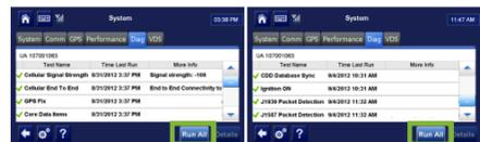
2. Confirm **✓** for Cellular Signal Strength, Cellular End to End, GPS, Core Data Items, Ignition ON, and CDD Database Synch. J1939 and J1587 are dependent on databus connections and mobile configuration set from VDC on portal.
