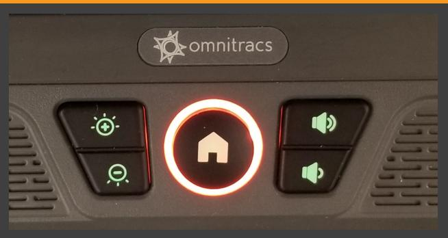
This shows the Intelligent Vehicle Gateway's (IVG) keyboard halo lit indicating that Unassigned Driving or a Diagnostics/Malfunction has occurred.
