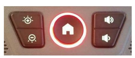
When messages are waiting or alerts are generated by applications on the ELD, the Home button has a colored Halo. The Halo remains lit until the message is read or alert is canceled/corrected. The Halo color represents the notification's importance.
